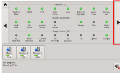
Interlock, Ignition, and Binary Inputs
